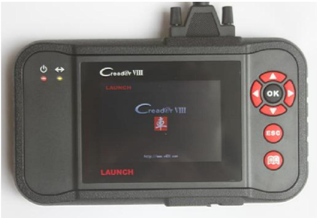
2Diagnostic Trouble Codes (DTC) that identify which section of the emission control system has malfunctioned
